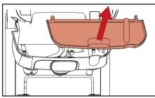
Fig. 5.11 - Remove internal drip tray
