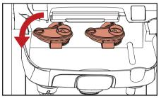
Fig. 5.10 - Remove mixing bowls
